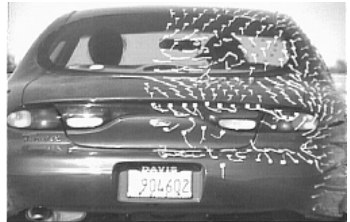
Figure 8. Tuft testing of stock 1996 Ford Taurus.
