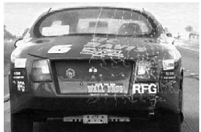
Figure 9. Tuft testing of UC Davis FutureCar.
